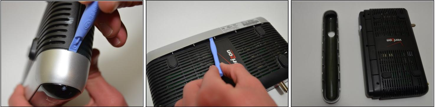
**⚠ Warning:** The design and location of the plastic clips holding this shroud make it extremely difficult to release. Take your time and use a second pry tool if necessary.
