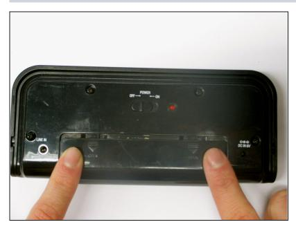
Use your fingers to slide the battery case cover off in the direction of the arrows.
