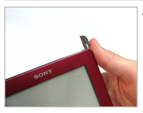
Remove the stylus from the device.
