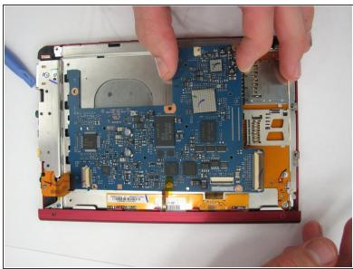
Lift the end of the motherboard closest to the memory cards and pull out.
