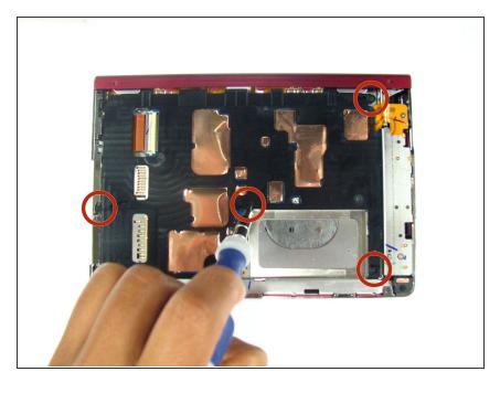
Using a screwdriver remove the four 1.4 mm screws that are holding the black plastic casing in place.
