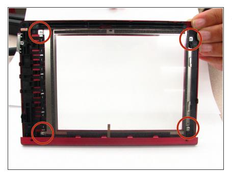
Using the Phillips head screwdriver, remove the four 1.4 mm screws holding in the plastic casing.
