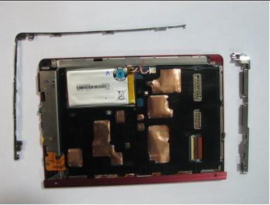
Pull the panel away from the device. You may have to use the flat end of the spudger to remove the side portion of the panel because it will be glued in place.
