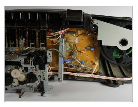
Carefully disconnect the wire connection by pulling at its base.
