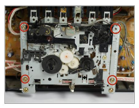
Unscrew the 3x12 screws circled in the photo using a #1 Phillips screwdriver.
