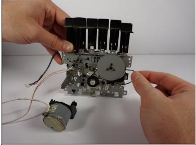
Remove the motor belt from its axle.
