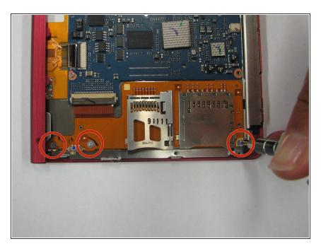
Using a Phillips head screwdriver, remove the three 1.4 mm screws located on the memory card holder.
