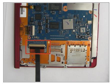
Using the flat end of the spudger, pry open the brown flap that connects the cardholder to the motherboard.
