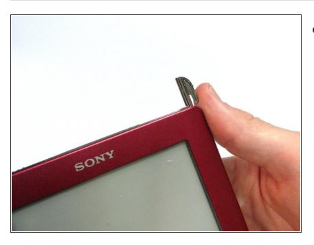
Remove the stylus from the device.
