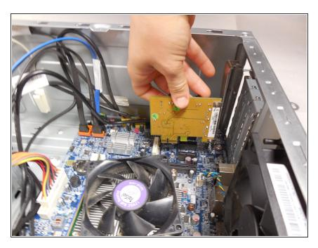
With moderate force, pull straight up on the expansion card to remove it from the computer.
