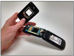
• With the plastic opening tool, work around the face plate until it pops off
