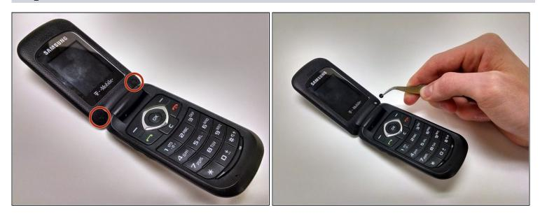
• Using the <u>tweezers</u>, remove the two rubber soles that cover the panel screws
