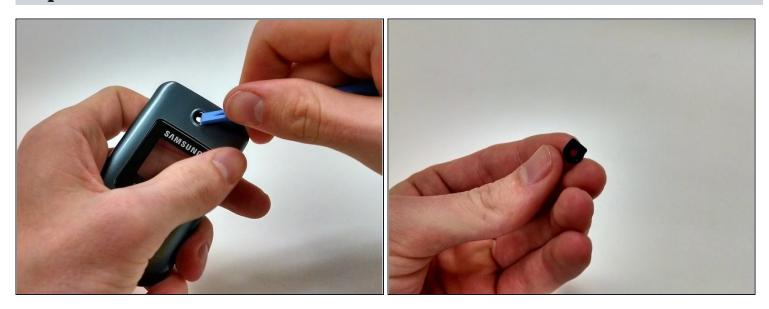
• Apply pressure to the lens, pushing it out the back
