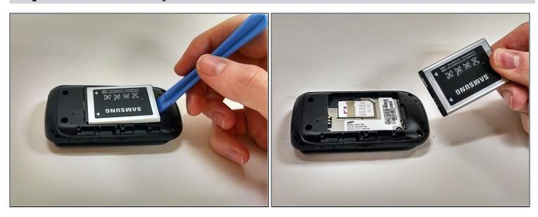
With a plastic opening tool, lift and remove the battery
