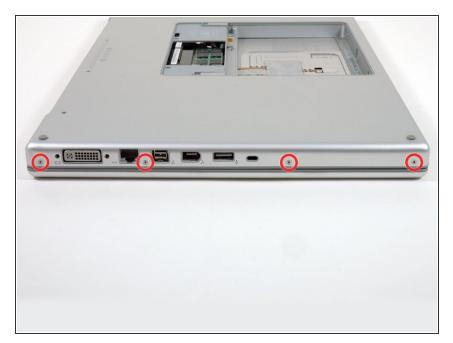
Remove the four 3.4 mm Phillips screws on the port side of the computer.
