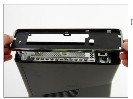
• Lift the top panel off the device.
