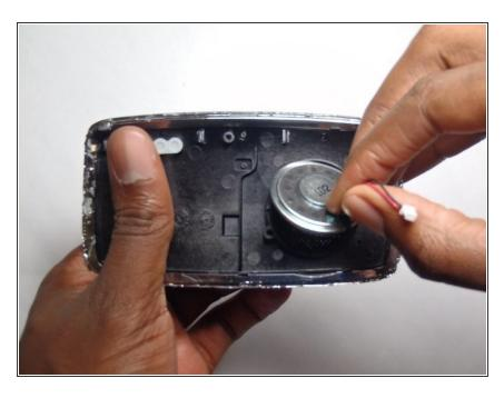
Gently pull the black and red wires away from the back plate to remove the speaker.
