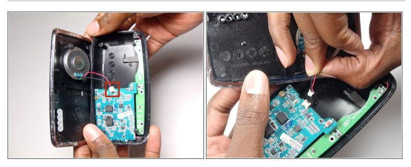
Carefully unplug the red and black wires that run from the speaker to the motherboard by detaching the white connecting piece.
