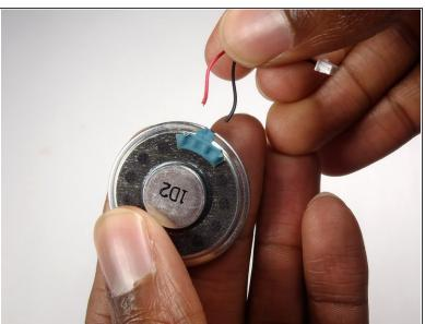
Carefully pull the wires away from the speaker, detaching them from the adhesive, while keeping the ends intact.
