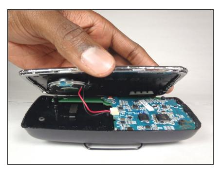
Open up the device by pulling the front plate straight up from the back plate.
