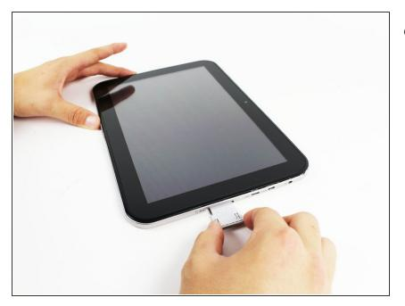
Remove the SD card from the SD card slot.
