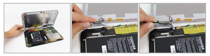
Remove the speaker cable from its socket by gripping both sides of the white connector piece with tweezers and pulling straight out.
