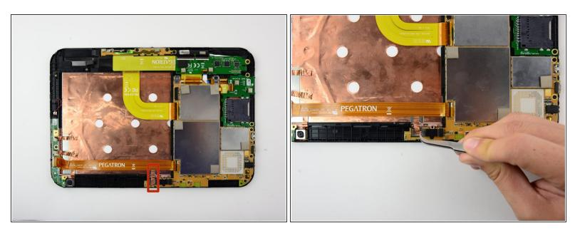
Using tweezers, pull the copper foil up from the back of the camera. It should peel up easily.
