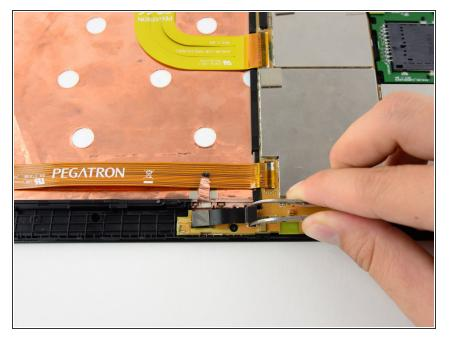
• Carefully remove the ribbon cable from the housing by pulling gently upwards on the sides of the cable housing. The cable should come straight up off of its housing.
