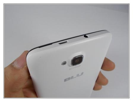
In order to remove the back case, start by flipping the phone to the back side and look at it from the top.
