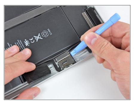
Use an iPod opening tool to release the SIM board from the adhesive securing it to the rear case.
