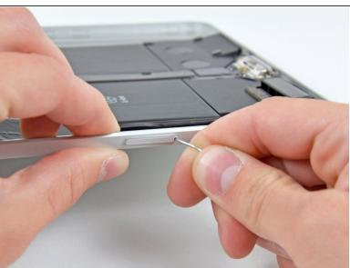
Insert a paperclip into the hole cut into the SIM card tray to eject it from the iPad.
