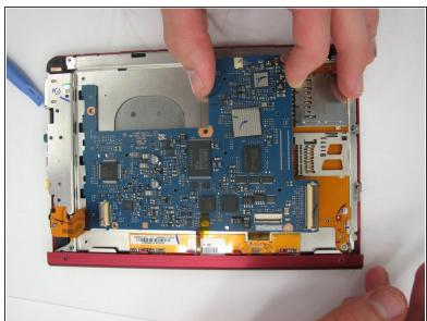
Lift the end of the motherboard closest to the memory cards and pull out.
