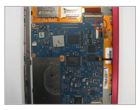
Using a Phillips head screwdriver, remove the one 1.4 mm screw holding in the motherboard.
