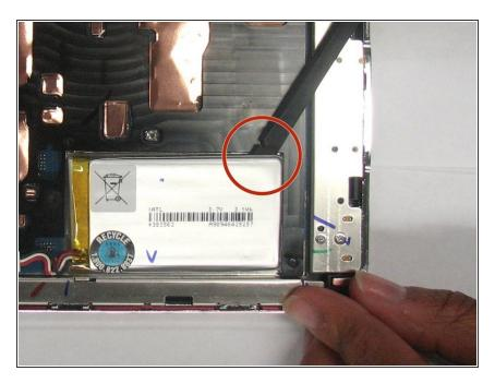
Use the flat end of the spudger to pry the battery out of its holder.
