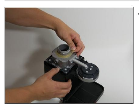
Grab the gasket and pull up until it is removed from the machine.
