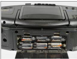
Remove the battery cover on the back of the boombox by applying downward pressure to the two clamps.
