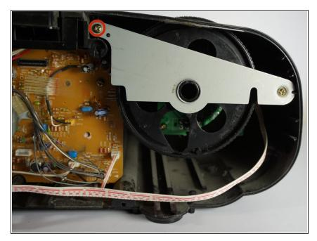
Use a Phillips #1 screwdriver to unscrew the 10 mm screw located on the top left of the tuner wheel bracket. Remove the metal bracket.
