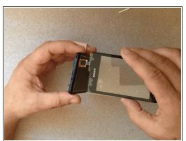
Install the new LCD into the frame and put adhesive tape.
