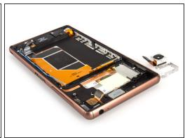
Remove front camera and rear camera.
