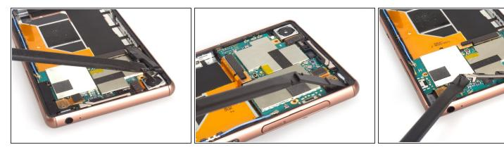
Remove three pieces of securing bracket.
