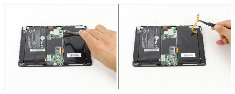
• Remove the battery connector using either your fingers or a pair of tweezers.
