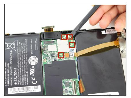
Lift all four <u>antenna connectors</u> from the motherboard again using the spudger.
