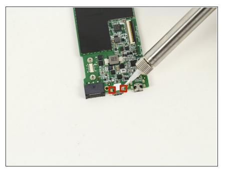
Use your <u>soldering skills</u> to detach the USB port from the motherboard at the following two solder joints.
