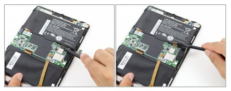
• With the spudger, remove the <u>flat-top connector</u> coming from underneath the motherboard.
