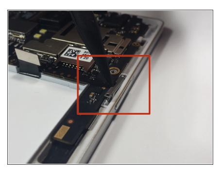
Use the sharp end of the spudger to pry the power button bracket from the side of the rear case.
