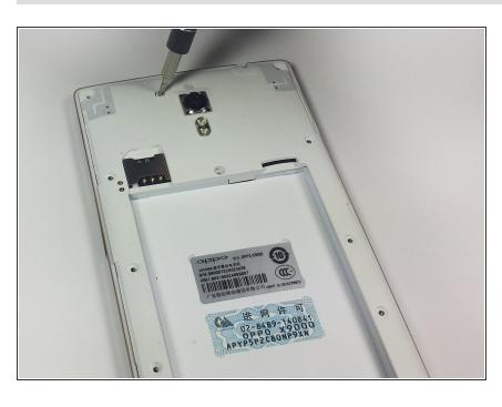
With the 3.6 mm Phillips screwdriver, remove the three newly exposed 3.6mm Phillips screws.
