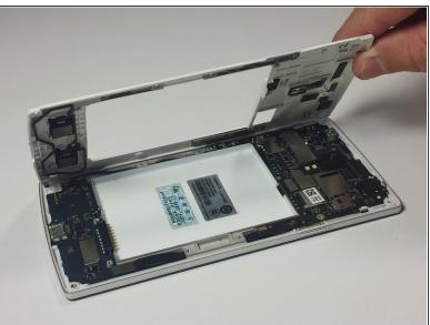
• Insert the plastic opening tool underneath the chassis near the power button and pry the chassis from the phone. This should take a little force.
