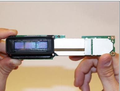
Using the spudger, detach the IR blaster board from the heatsink.
