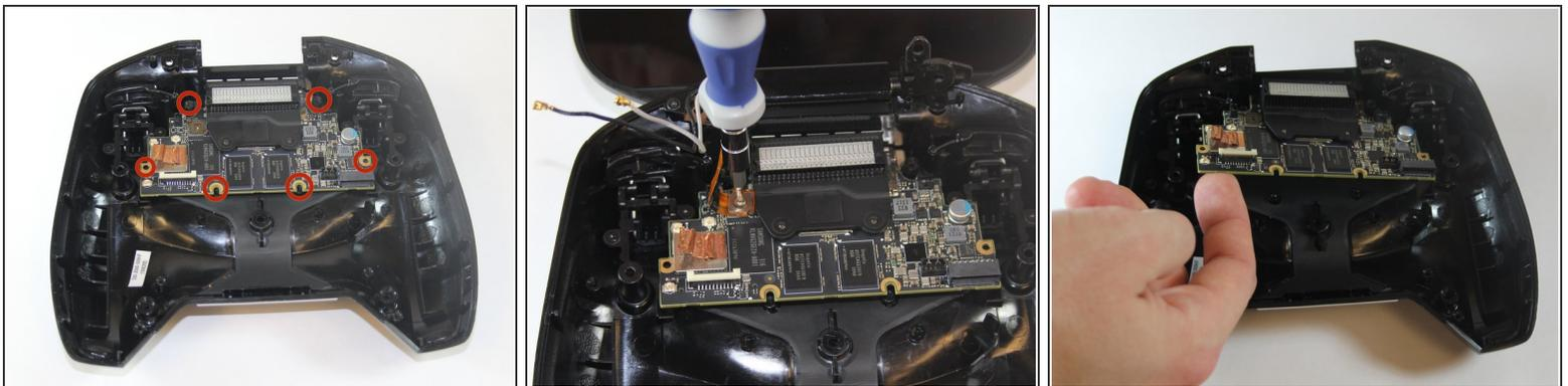
**i** The large board under the back case is the motherboard.
