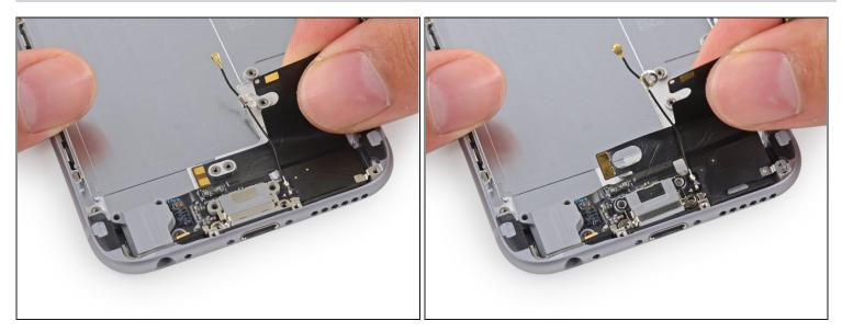
• Carefully pull the Lightning connector cable assembly up slightly to free the it from the vibrator and speaker screw posts.
