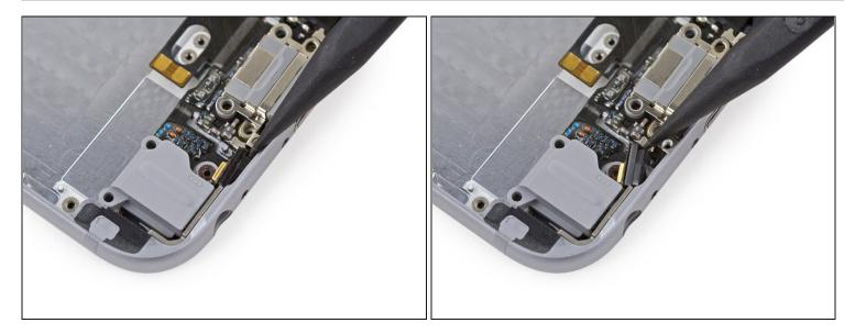
• Use the point of a spudger to push the microphone portion of the Lightning cable assembly out of its recess in the rear case.
