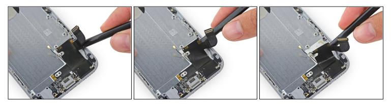
• Use the flat end of a spudger to begin peeling the Lightning connector cable assembly up from the rear case.
