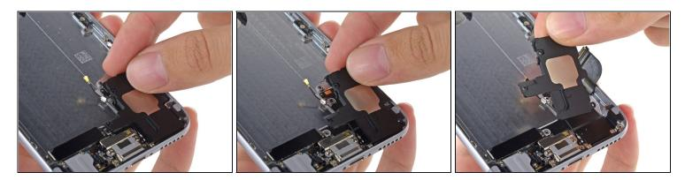
• Pull the speaker up and out of the rear case.
