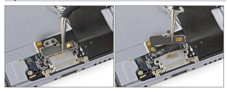
• Remove the Lightning port retaining bracket.
