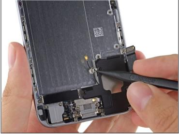
Use the point of a spudger to push the antenna interconnect cable clip off of the speaker housing.
