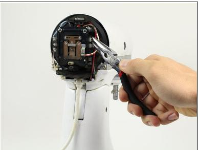
Using pliers, remove the connections for each of the four wires connecting to the circuit board.
