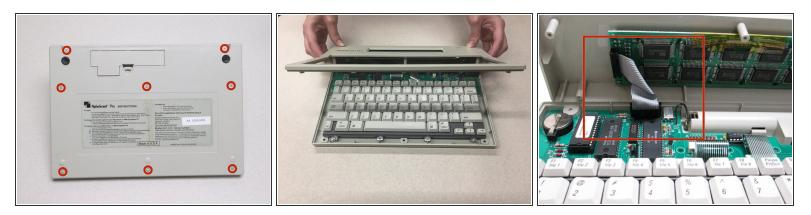
A Power off your AlphaSmart Pro device and remove the batteries before beginning disassembly.
