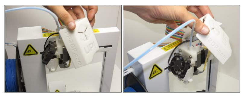
Remove the plastic cover that sits on the extruder, next to the fan, by lifting the latches in the back.
