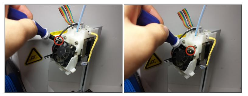
Using the Phillips #0 screwdriver, locate and remove the two 3mm screws on the top of the fan using a counter-clockwise rotation.
