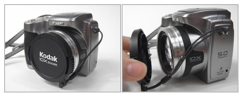
Remove lens cover from the camera by squeezing the protruding button on each side of the cover and pulling.
