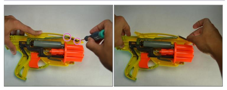
• Using a screwdriver, remove the 7.5 mm phillips 00 screw holding the top spring to the reload slider.
