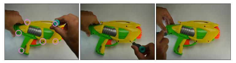
Using a screwdriver, remove the six 9 mm phillips 00 screws holding the main body together.
