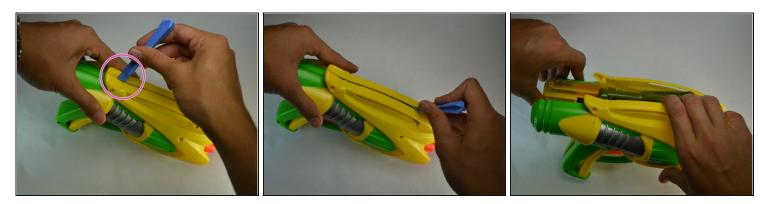
Using the plastic opening tools, carefully take apart the main case of the blaster to leave the inside exposed.
