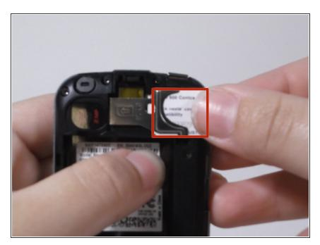
• Locate and use your thumb to slide the SIM card to the right until it is removed and set it aside.
