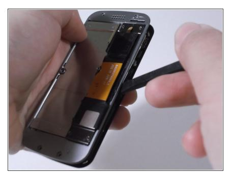
Insert the flat end of a Spudger in between these two pieces of the phone and move it along the sides to loosen and pry apart.
