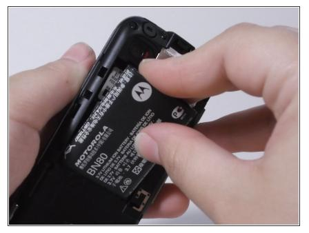
Locate battery and use your index finger to grasp the upper left side of the battery and pull back to remove. Set battery aside.
