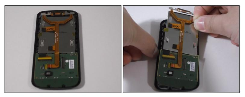
• Peel back the yellow tape on the side of the screen using tweezers or your fingernails. Lift away screen and board.
