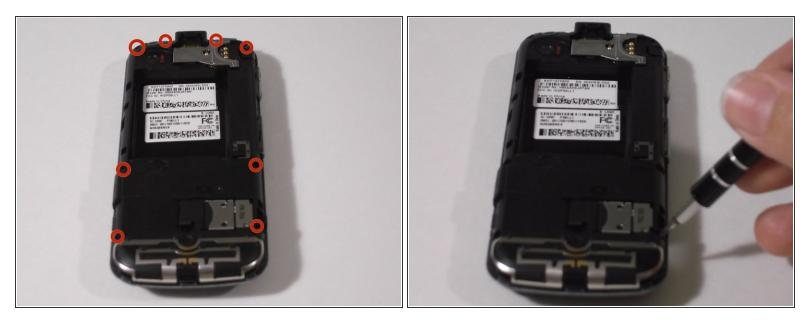
Remove eight black .4 centimeter screws on the top, bottom, and sides of the phone with a T5
