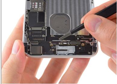
Grasp the antenna connector with a pair of tweezers and gently lift it from its retaining clip on the logic board.
