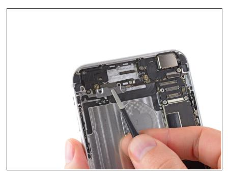
Grasp the antenna bracket with a pair of tweezers and lift it off the iPhone.
