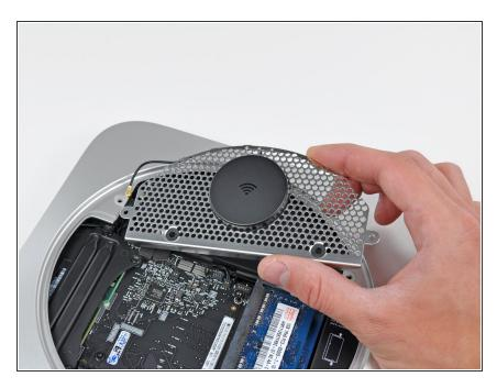
Remove the antenna plate from the mini.
