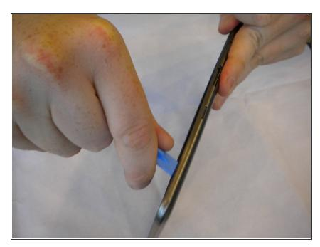
Slide the second plastic opening tool along the edge of the device to separate the back cover from the screen.
