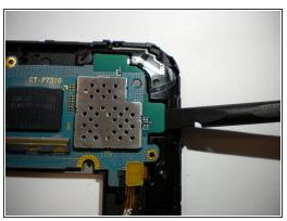
Using the flat edge of the spudger, pry and lift up the motherboard.
