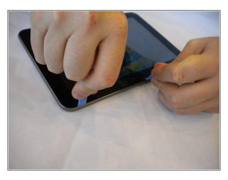
6 cm [2 in] away from the first plastic opening tool, insert a second plastic opening tool between the back cover and the screen.
