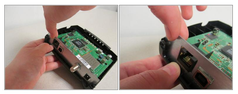
After opening the router, grab the upper left corner of the sliver face plate and gently pull the motherboard out of the slot from within the case.
