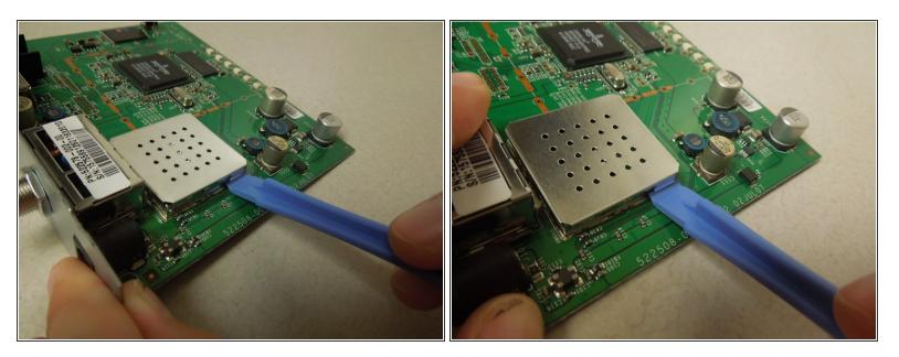
Holding the motherboard by the metal face plate, position the flat end of a prying tool under one of the prongs of the metal square plate.
