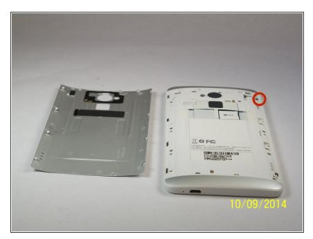
Lift back cover while pressing highlighted release switch towards the center of the phone.
