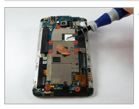
Remove the seven 3 mm Phillips #000 screws from the motherboard.
