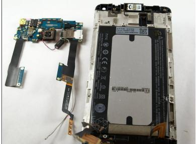
Lift the secondary motherboard with the camera attached.
