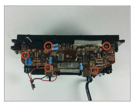
Remove the top 5 10mm Phillips #1 screws holding the top part of the motherboard
