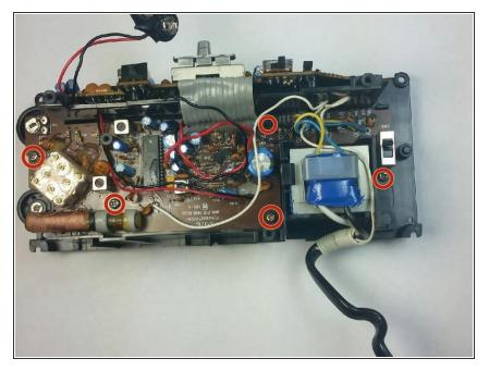
Remove the 5 10mm Phillip's #1 screws that holding side part of the motherboard
