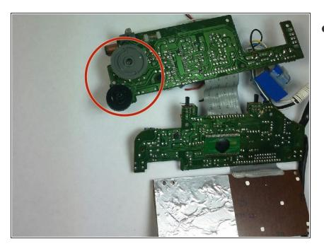
Tuning wheel, lift it up and replace it with a new one.
