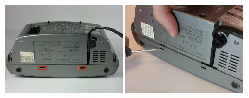
• Using flathead screwdriver undo the release tabs.
