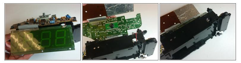
• Remove the motherboard from the frame using the illustration shown.
