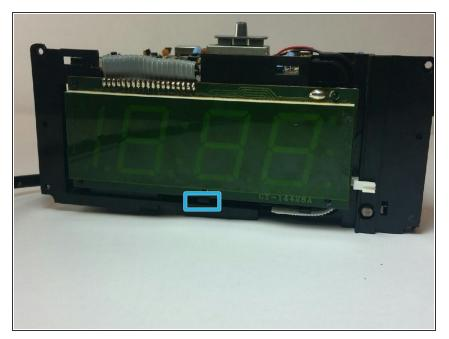
• First release the latch highlighted in the picture. Then grab the screen by the bottom and lift it up.
