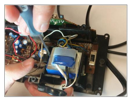
• Remove the transformer by pulling back the release tab shown.
