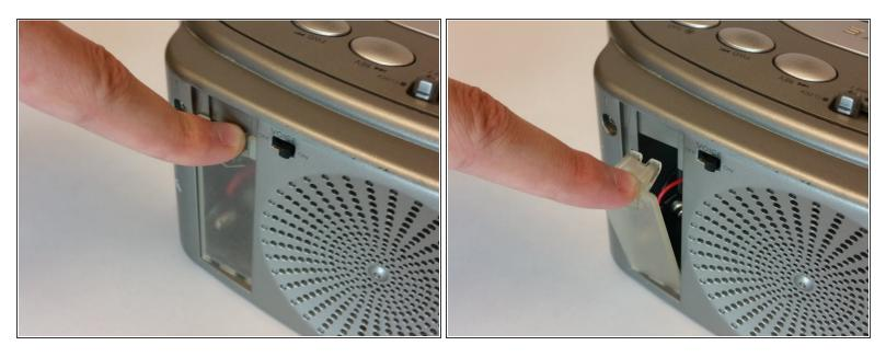
• Push down on the clip to release pressure. The pull off the plastic cover.
