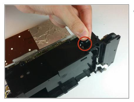
• Pull the battery terminal through the whole shown.
