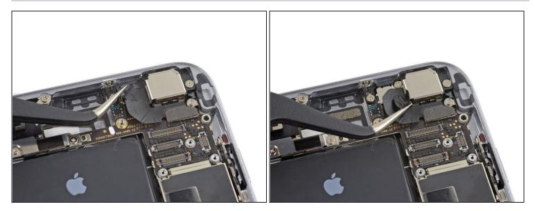
• Remove any tape covering the upper left rear-facing camera screw.
