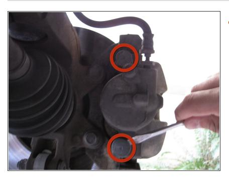
Use a flat head screwdriver to remove the black plastic guide bolt dust caps.
