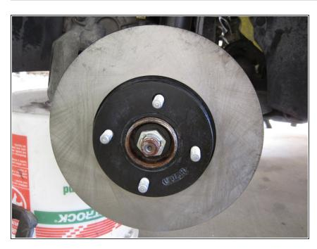
Install the new rotor over the wheel lugs.
