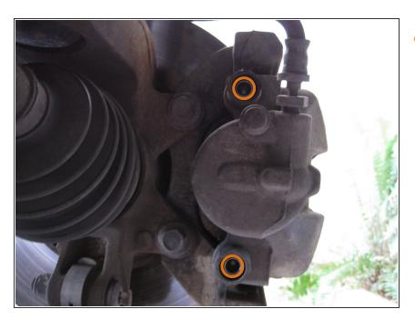
Use a 7 mm Allen wrench to remove the two caliper guide bolts.
