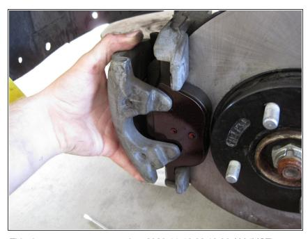
Place the caliper back on the rotor.
