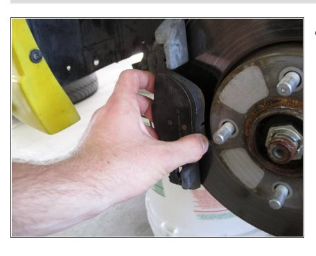
Pull the outer brake pad from the mounting bracket.
