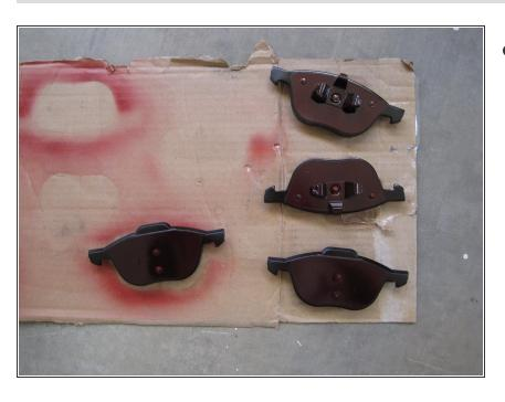
Coat the steel backing plates of the new brake pads with an anti-squeal coating.
