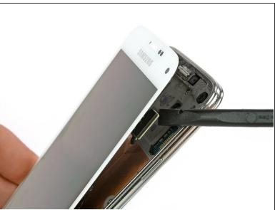
Neep the top portion of the display assembly next to the frame.
