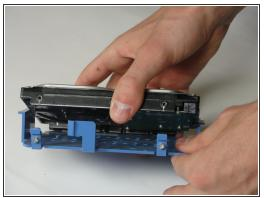
Pull the 2 blue tabs away from the hard drive and then pull the hard drive case down.
