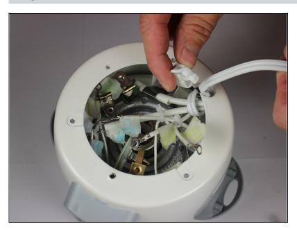
Locate the small white latch on the side of the knob and pull it away from the cord. This will unlock it and expose he cord underneath. Set the knob aside.
