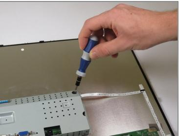
Unscrew the four 7.5 mm Phillips #2 screws connecting the motherboard to the metal casing.
