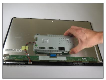
• Gently lift the motherboard casing from the monitor.
