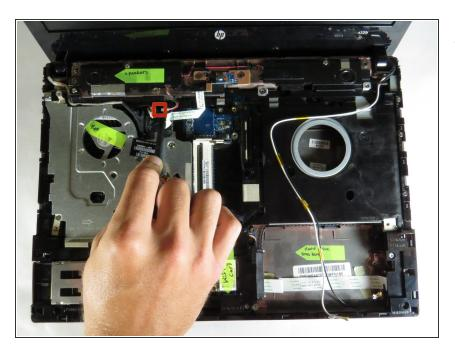
Use the black spudger tool to lift the white, black, and red ribbon cable connector up so that it is disconnected.
