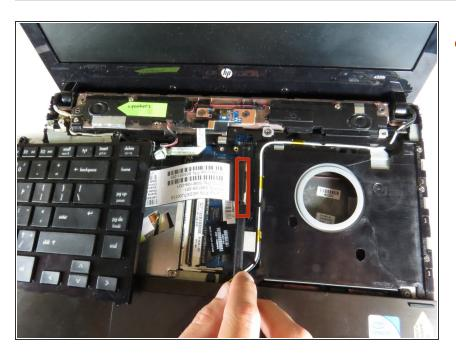
Use the black spudger to lift the black latch holding the keyboard ribbon cable.
