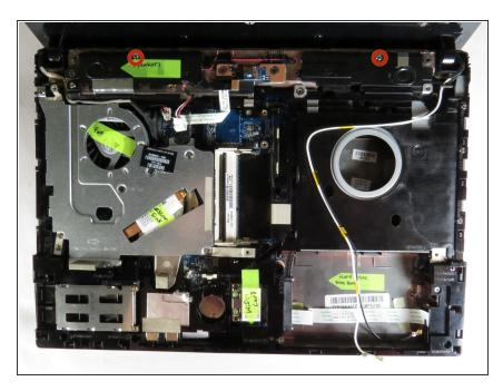
Unscrew the two (2.5 mm Phillips) screws (located on the upper most part of the computer) holding the speakers in.
