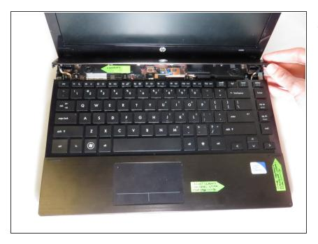
Slightly push up while lifting up on the power button panel to release the panel.
