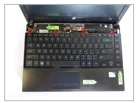
Unscrew the four (2.5 mm Phillips) screws holding the keyboard in (Use Phillips #0 Screwdriver).
