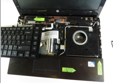
• Carefully (holding both sides of the keyboard), push up and lift slightly.
