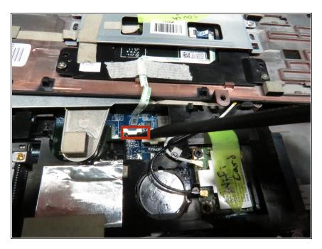
Using the black spudger, slightly pry up on the ZIF connector and lift out the wire carefully.
