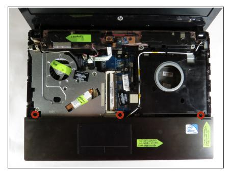
Unscrew the three (2.5 mm Phillips) screws holding the bottom touchpad panel.
