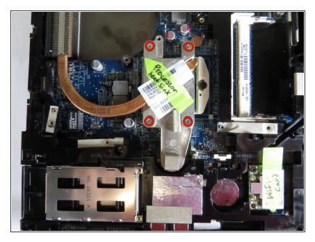
Unscrew the four (2.5 mm Phillips) screws holding the processor heat sink in (located near the center of the laptop)
