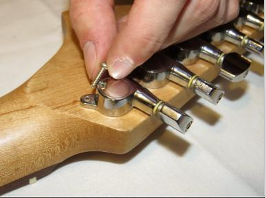
Next, remove the screws from the backside of each tuner.
