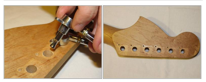
• Finally, remove the tuning machine assembly from the headstock.
