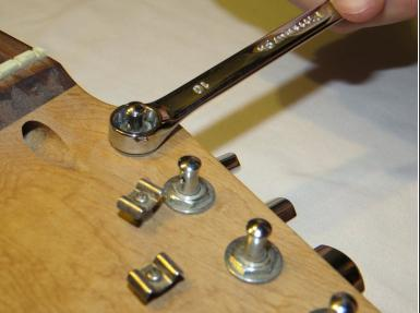
Using a wrench, remove the nuts around each tuning head post.
