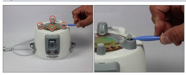
Each of the four legs has a rubber cushion on its bottom. For each cushion, insert a plastic opening tool between the plastic leg and rubber cushion, and pry off the rubber cushion.
