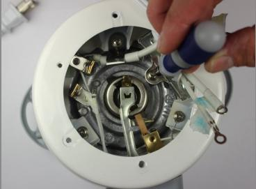
Unscrew the four 10 mm long 7mm diameter Phillips screws attached to the hotplate
