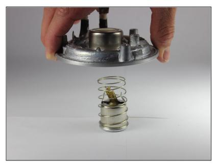
Remove the non-spring portion of the hotplate by lifting it up, exposing the spring and brass locking latch underneath.
