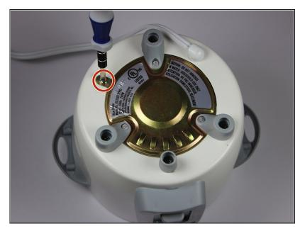
Using a spanner screwdriver, remove the one 10mm long 7mm diameter spanner screw from the side of the brass panel.
