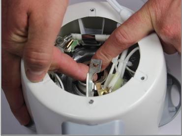
• Using a pair of pliers, bend the spring latch from a "[" shape to a "c" shape so that it fits through the silver-colored latch that holds it. Then pull the silver-colored beam up so that it detaches from the brass beam.
