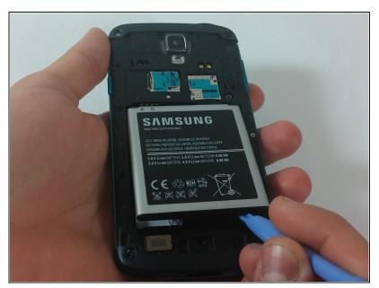
Insert a plastic opening tool, or your finger, into the notch of the battery compartment and lift the battery upward to remove it.
