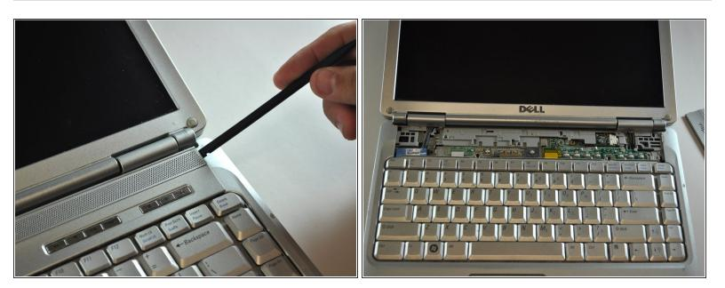
Using a spudger, pry off the top cover plate, thus exposing the screws for the keyboard.
