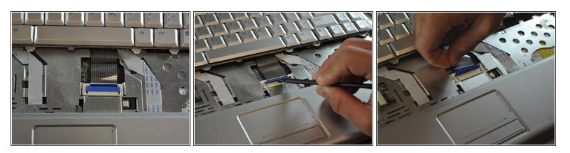
Using a spudger, carefully lift the blue tab, releasing the ribbon connector and freeing the keyboard to be removed.
