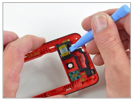
• Use an iPod opening tool to pry the rear speaker out of its housing in the rear inner frame.
