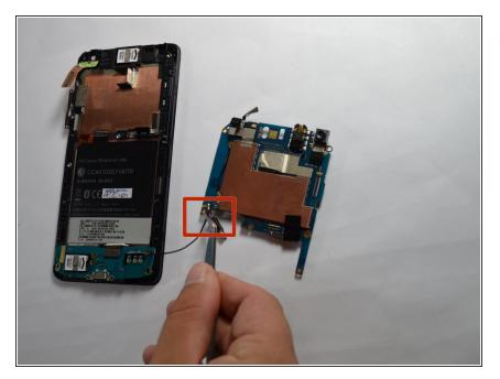
Unsnap the wire from the printed circuit board (PCB) using the tweezers.
