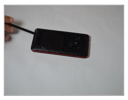
• Use spudger tool to pry under the battery to lift it up and out.
