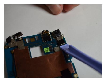
• Remove the camera using the plastic opening tool as shown.
