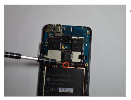
Remove the 3mm PH00 screw located at the bottom center of the motherboard using a P#00 Phillip's head screwdriver.
