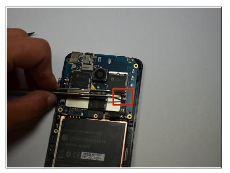
Using the tweezers gently disconnect the wire from the vibrator located on the motherboard.
